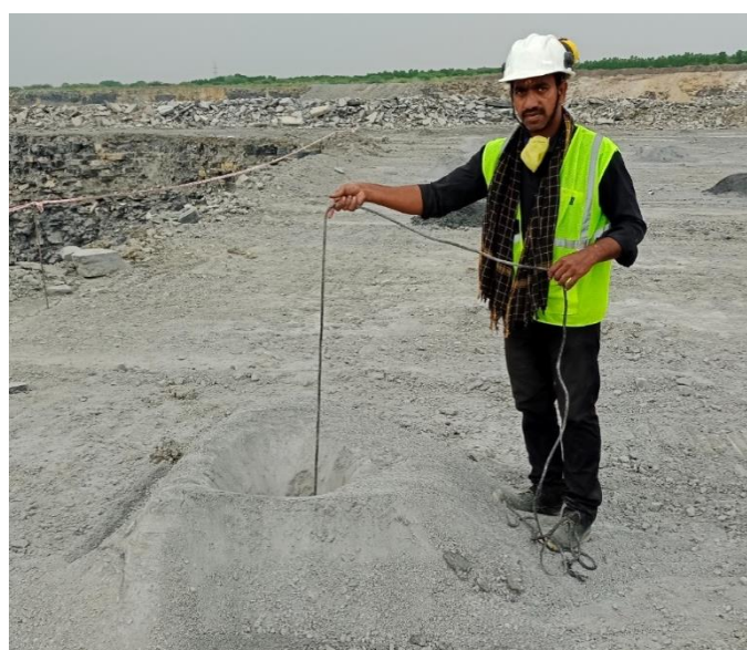
Fig. 4: Hole measurement taken to maintain an optimal level of 10m depth
