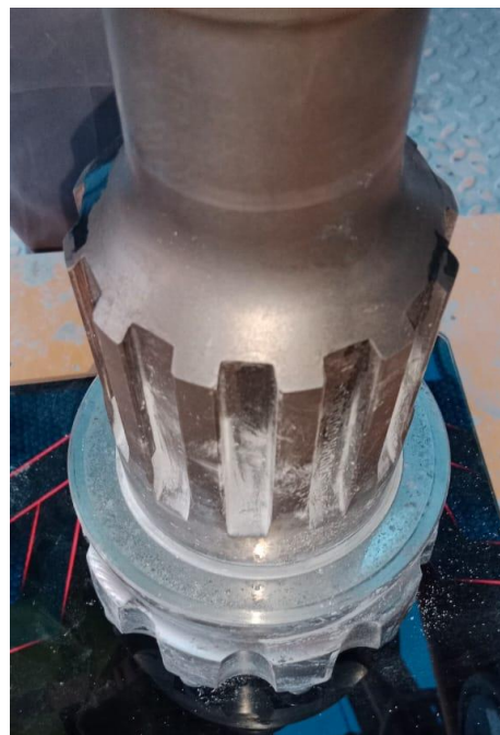
Fig. 1: 165mm Drill bit used in present study
